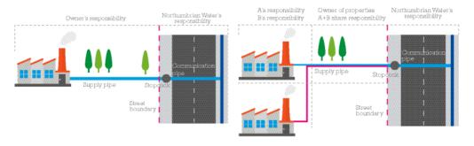
The two diagrams have been set out to show examples of property boundaries and responsibilities. The diagram on the **left** shows which pipes belong to us and which belong to your non-household customer. The diagram on the **right** shows an example of a shared supply.
