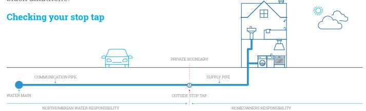
Black Alkathene pipework was often used as the supply pipe to properties in the 1960, 70s and 80s. As you can see on the picture above, the pipe connecting properties to the water main is composed of two sections - the communication pipe and the supply pipe. The section running from the water main to the private boundary is called the communication pipe and is the responsibility of Northumbrian Water. The section running from the private boundary (usually from the external stop tap)
