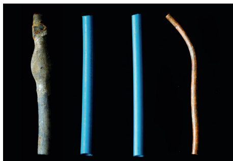
In order from left to right: lead, specialist barrier pipe (copper and plastic), plastic, copper.
